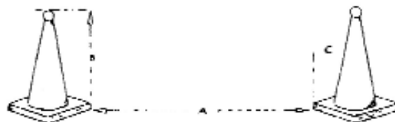
Placement and Measuring width of cones
